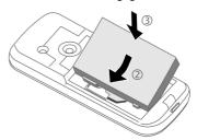
To remove, press the retaining tab on the side of the battery, then lift the battery out.  Place the battery cover on the phone slightly off centre
