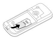
Insert the battery sideways into the phone ②, then press it downwards ③ until it engages.
