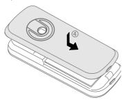
To remove, press the battery cover ⑤, and slide it off the phone ⑥.
