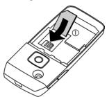
Insert the battery sideways into the phone ②, then press it downwards ③ until it clicks into position.
